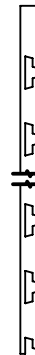
1 HALF GROOVE Square end on one side and half groove on the other for stacking
